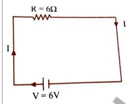
(b) Electrons give up energy at the rate of  $RI^2$  per second to the thermal energy. What time scale would one associate with energy in problem (A)? N = number of electron/volume =  $10^{29}$ /m<sup>3</sup>, length of circuit = 10 cm, cross-section A = (1mm<sup>2</sup>)
